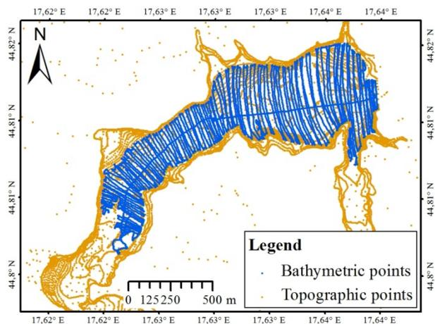
Figure 5. Location of bathymetric and topographic survey points in Drenova reservoir and the accumulation area.
