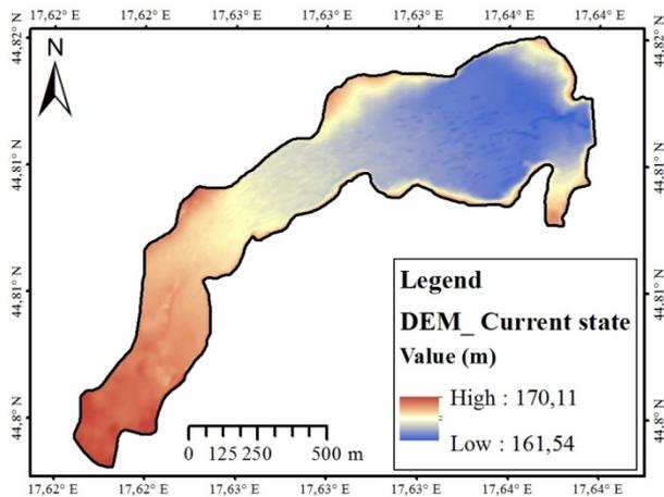
Figure 6. Digital elevation model (DEM) of Drenova reservoir from 2012 - current state
