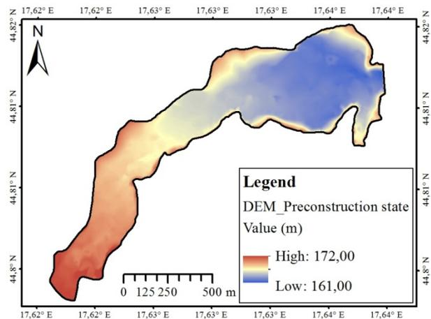
Figure 4. Digital elevation model (DEM) of Drenova reservoir from 1978 - preconstruction state
