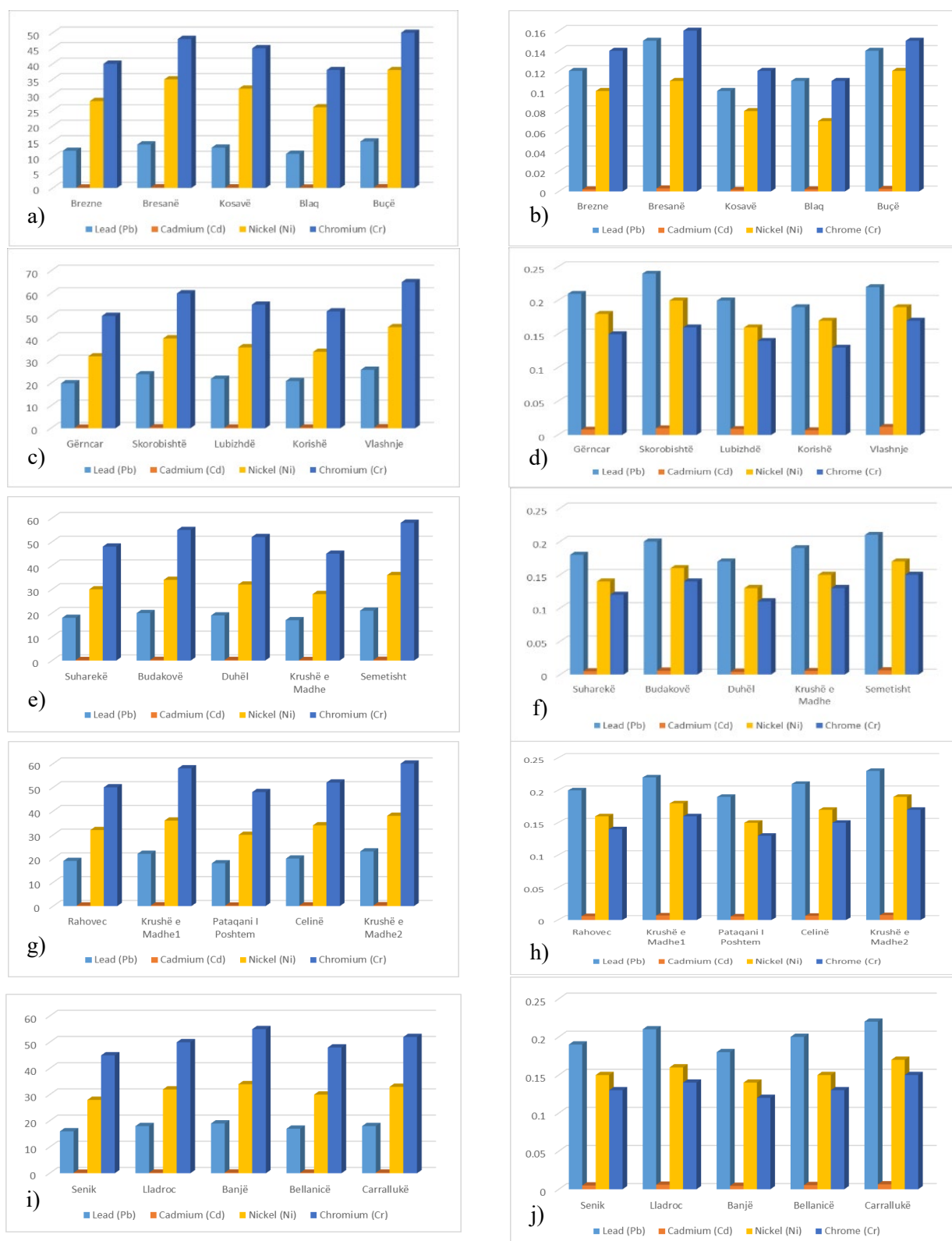
Figure 3. Results of heavy metal concentrations (mg/kg) in soil (a, c, e, g, i) and cabbage (b, d, f, h, j) across the municipalities of Dragash, Prizren, Suharekë, Rahovec, and Malishevë, respectively.
