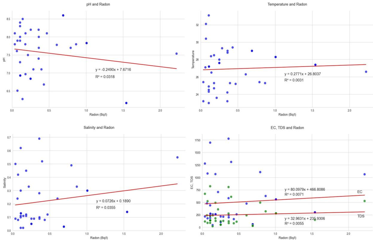
Figure 4. Graph showing the relationship between the properties of various water sources and radon concentration.
