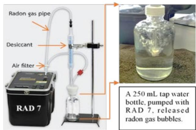
Figure 2. Radon gas measurement in tap water samples using RAD H<sub>2</sub>O.
