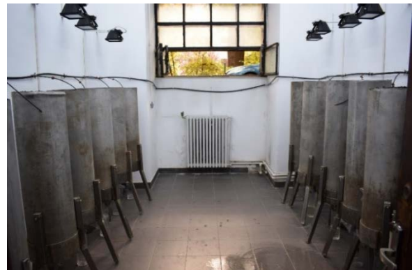
Figure 4. Water infiltration under flooding in the soil columns set above the stainless circular holders provided with drainage systems in the laboratory and collecting the effluent in bottles
