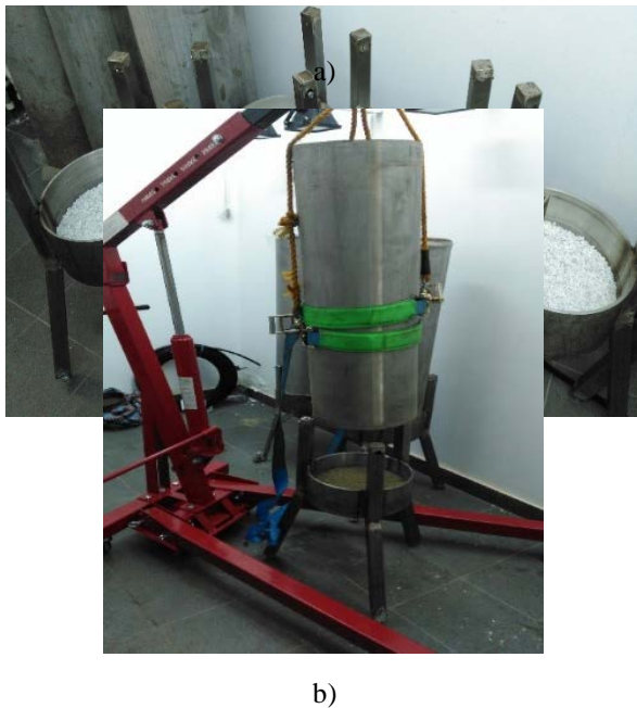
Figure 3. Stainless steel circular holders provided with the lower drainage layer, a 3-7 mm sized gravel (a), the crane manipulating a soil column with tow fastening belts above a holder with both drainage layers – the upper one seen, the sand (b)
