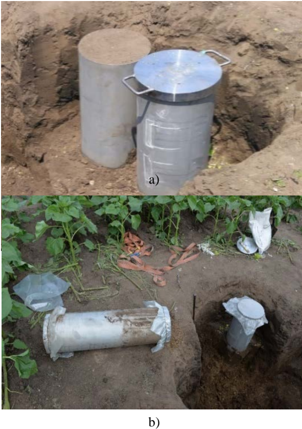
Figure 2. Sampling undisturbed soil columns by using a sampling steel cylinder above for pressing or hitting (a) and binding the ends of columns with double-layer plastic sheets (b)
