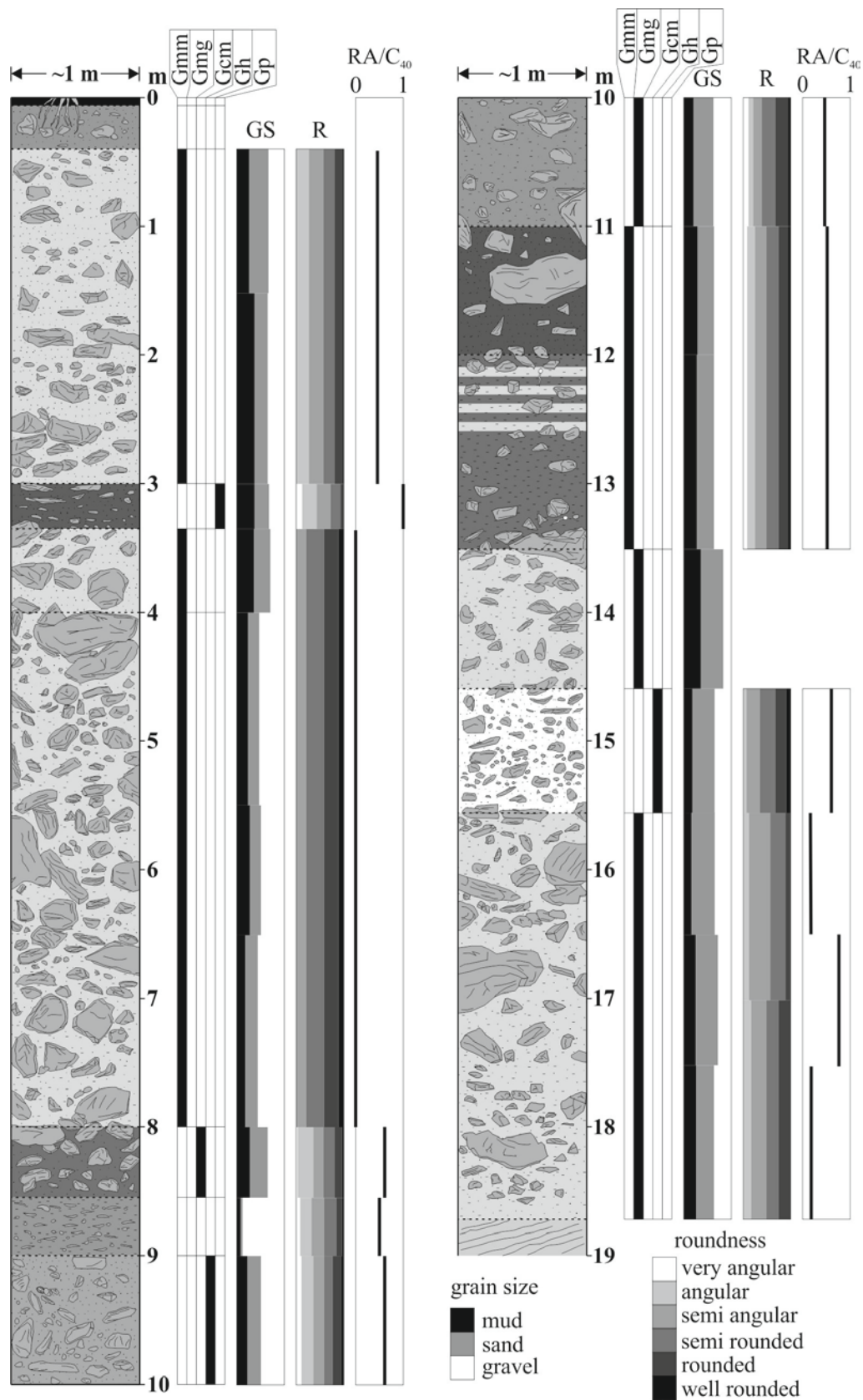
Figure 7. Facies distribution and composition of the outcrop in the site C. The grain size (GS) and roundness (R) are expressed as a percentage of the analysed fraction and roundness category, respectively.
