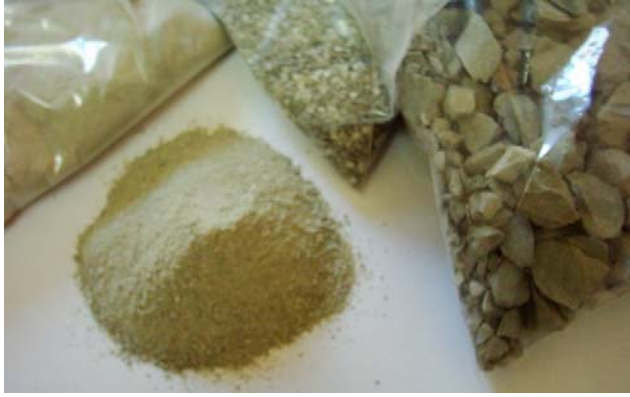
Figure 2. Zeolitic tuff crushed and milled at < 1 mm particle size range
