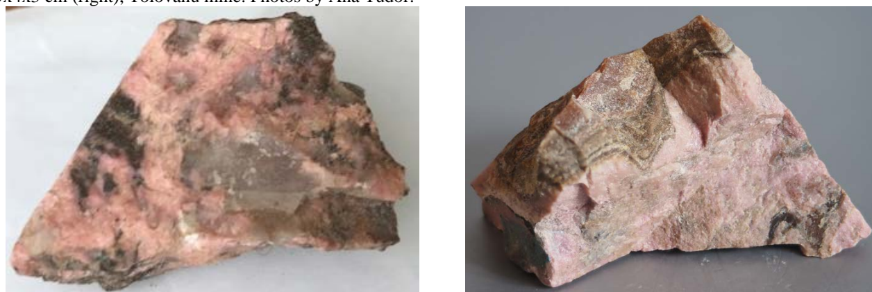
Figure 3. Natronambulite (pinkish orange), celsian (centre and left bottom, white), Li-amphibole (greenish black, left middle) sample BTm420, 6x6x3 cm (left); Rhodonite (light rose), banded by aegirine –acmite /serandite/ ardennite association (top, yellow-brown), sample BT258R, 5x3x4 cm (right), Tolovanu mine. Photos by Ana Tudor.
