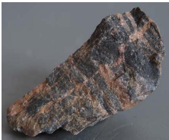
Figure 6. Braunite rich band (black) cut by natronambulite (light orange) veinlets, sample BT1002C, 6x3x2 cm (left); Hausmannite (brown “chocolate”) relics in nambulite ore (orange) and cut by very small nambulite veins, sample BT262, 3x3x2 cm dimensions (left). Photos by Ana Tudor.
