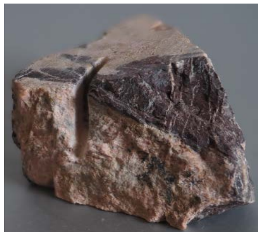
Figure 6. Braunite rich band (black) cut by natronambulite (light orange) veinlets, sample BT1002C, 6x3x2 cm (left); Hausmannite (brown “chocolate”) relics in nambulite ore (orange) and cut by very small nambulite veins, sample BT262, 3x3x2 cm dimensions (left). Photos by Ana Tudor.
