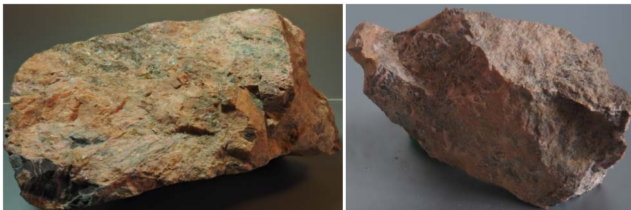
Figure 1. Coarse orange nambulite crystals of 2 cm long, leakeite (greenish yellow, middle top), braunite-bixbyite (black, small, bottom, left), sample BT250, 12x6x6 cm, Tolovanu mine (left); Large yellow pinkish natronambulite (centre) banded with rich acmite-aegirine (violet brown), sample BT1001, 14x10x8 cm (right). Photos by Ana Tudor.
