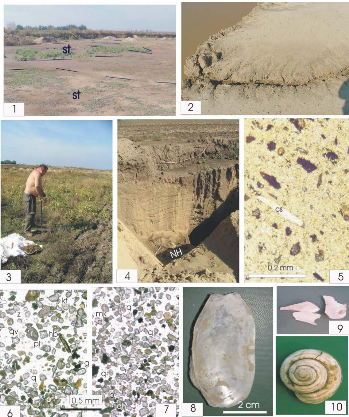
Photo 1: View of excavation, showing the grass covered silty and the uncovered sandy-silty Pleistocene sediments. Photo 2: Outcropping sodic clay with branched erosional trenches leading to the pluvial pond on the left side of the picture. Photo 3: Géza Kutasi drills the Ejk-2 shallow borehole. Photo 4: The main dug well with ancient hydrostatic level (NH). Photo 5: Micrograph of lime concretion from 74. measured section. In micritic carbonate background, small pores and a crushed snail piece (cs), thin section, \parallel nichols. The sand fraction of Pleistocene samples (photo 6) and Holocene samples (photo 7) q, quartz; qv, volcanic, hemihedral quartz; kf: potassic feldspar; pl, plagioclase; b, biotite; hb, red hornblende; e, epidote; g, garnet; z, zircon; t, titanite; l, limonite; p, slightly limonitized pumice; mk, micritic lime concretion; ch, chloritic schist fragment. Photo 8: Unio pictorum L., whole shell. Photo 9: Unio splinted shell fragments. Photo 10: Cypaea hortensis (Fér.) shell.
